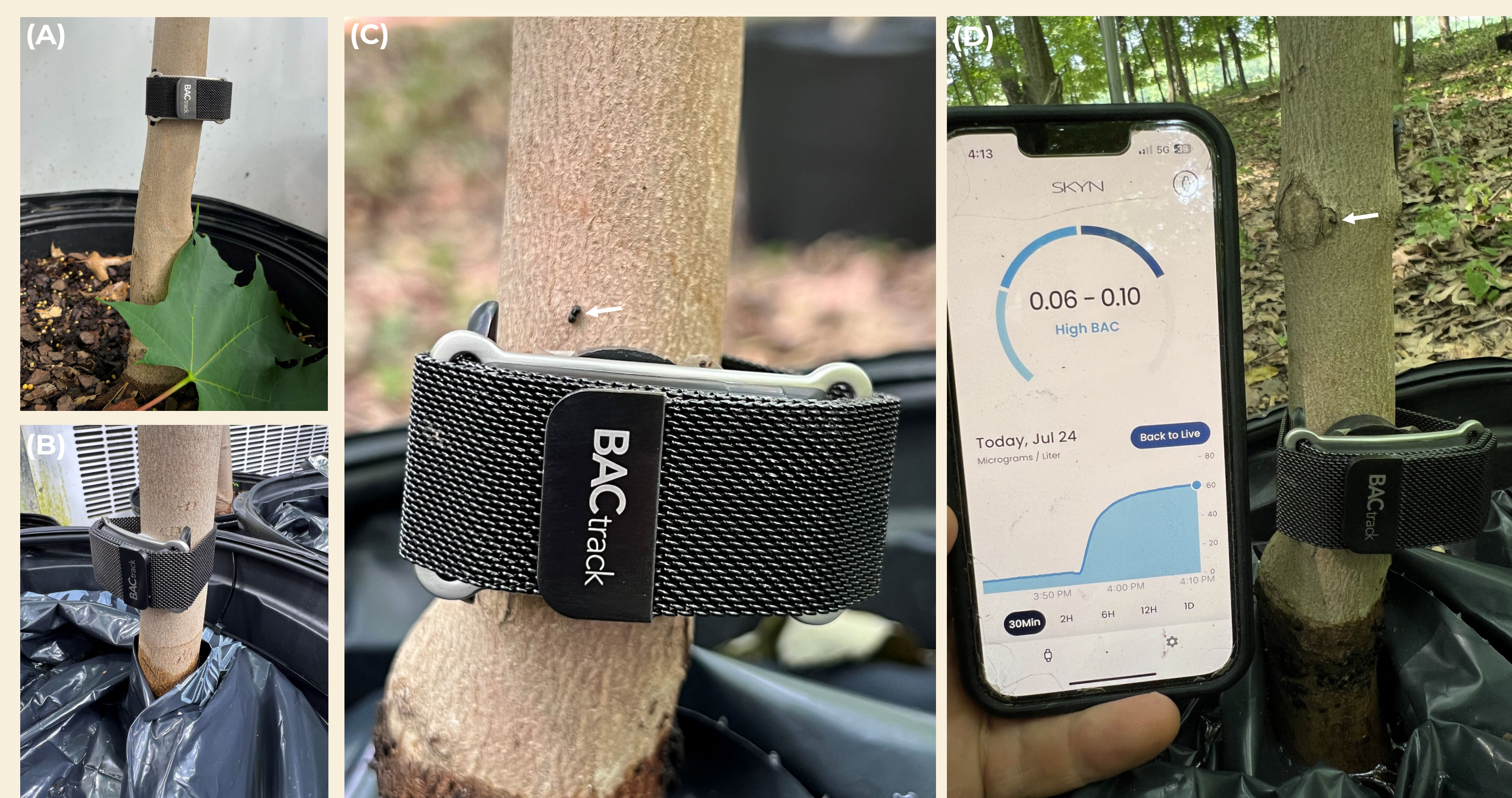
Fig. 1. BACtrack ethanol biosensor attached to sugar maples subjected to (A) standard irrigation and (B) flood stress. (C) Ambrosia beetle (arrow) and BACtrack biosensor on a flood-stressed sugar maple stem. (D) Transdermal alcohol content ( \mu\text{g/L} ) recorded in near real-time from a flood-stressed sugar maple tree as an ambrosia beetle has initiated tunneling (arrow).
